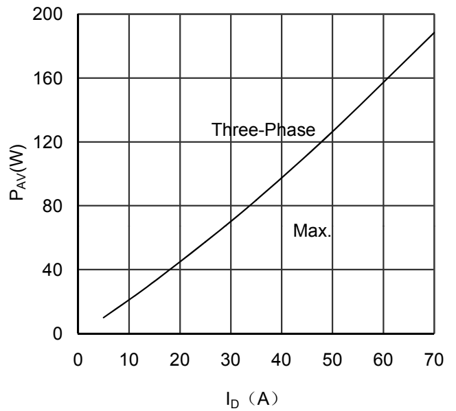
Figure 2. Power dissipation vs Output Current
